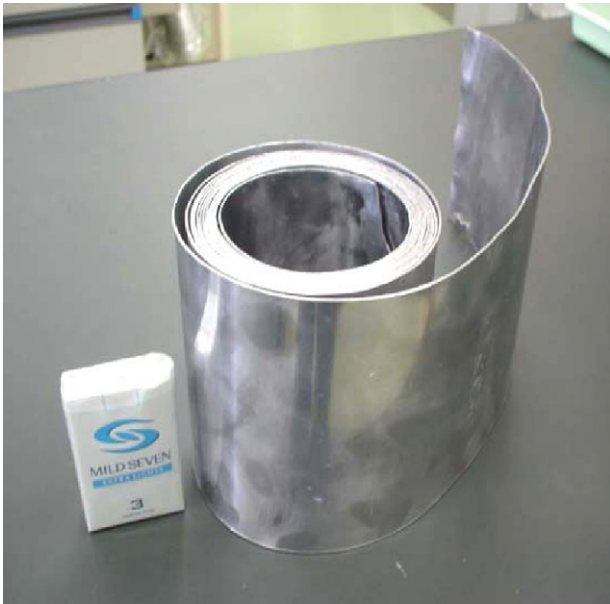
Fig. 4. 1.5 wt%Sn lead alloy sheet wound up by the test powder roll machine.
